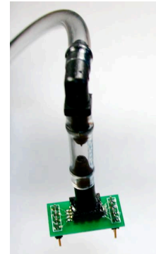
Figure 2c Pressure sensor with tube coming from water measurement column.
