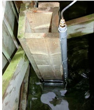
Figure 2b Water measurement column with tube leading to pressure sensor.
