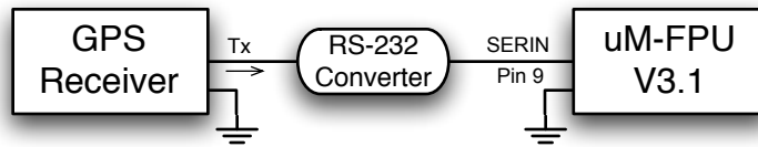
Figure 1: Connecting a GPS Receiver to the uM-FPU V3.1 chip
