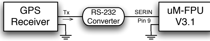
Figure 2: Connecting a GPS Receiver to the uM-FPU V3.1 chip
