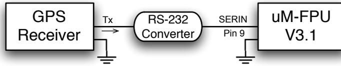
The serial output from the GPS receiver must be an NMEA data interface running at 4800 baud. Figure 3 shows sample output from the program.
