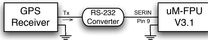
Figure 2: Connecting a GPS to the uM-FPU V3.1 chip.
